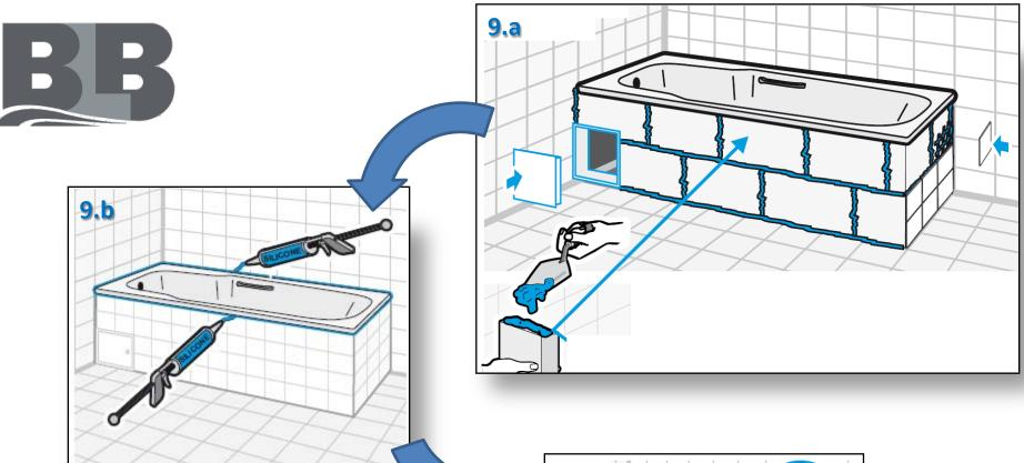
9. When building the surrounding wall be sure to allow for an access to the wastepipe valve. All the points of contact between the bathtub and the side walls should be done with silicone. The bathtub should only be used after 24h.
