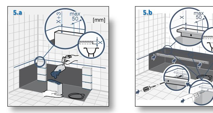
5. The bathtub should be sustained mainly on the sides against the wall. The installer can choose to sustain in brickwork (5.a), by means of an outline or metallic tube or with a wooden beam fixed to the wall (5.b).
